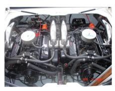
Unfortunately the starboard side engine block cracked on me and I replaced that engine with a matching 454 again.
